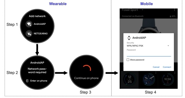
Figure 2: Example of the inter-device communication between a wearable and a mobile device. The setup of a WiFi connection starts in the wearable, but then the process continues on the mobile due to the difficulty of typing the password on the wearable device.
