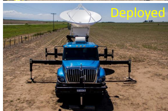
Figure 8. COW assembly. COW as transported, antenna being assembled, antenna lifted onto pedestal, deployed.
