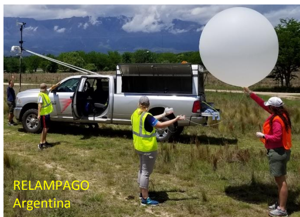
Figure 12. FARM MQD sounding being launched from an MM which also carries PODNET units.
