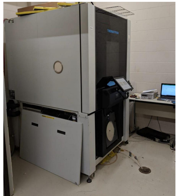
Fig. 1 Environmental chamber: Thermotron SE-600-10-10
