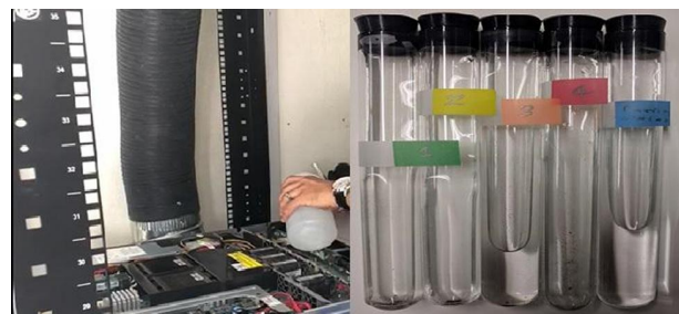
Fig. 7 Collected dust samples from server chassis
