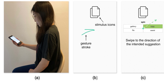
Figure 5: (a) A user is inputting the command “copy” with BackSwipe. (b) The stimulus icon is displayed on the front screen. (c) The decoder shows the command “spin” with four more candidate commands. Since “spin” is not the intended command, the participant swipes her finger to the direction of the intended word “copy” as if the finger is located at the center of the suggestion grid (i.e., top-right direction). In other words, drawing a gesture towards top-right corner would select the “copy” command
