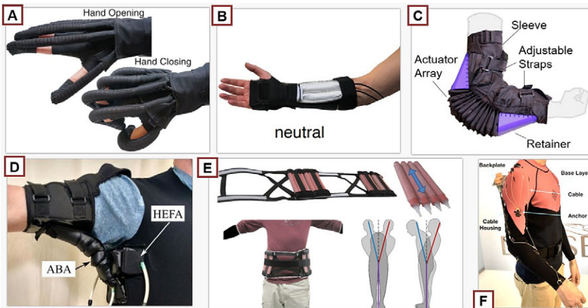
Figure 5. A brief survey of recent soft wearable robot (SWR) technologies for each of the following upper body joints: (a) a soft robotic hand developed at Harvard University at the Wyss Institute for Biologically Inspired Engineering (Cappello et al. 2018b), (b) a soft assistive device for the wrist made from fabric materials (Realmuto and Sanger 2019), (c) a soft elbow exosuit designed at Arizona State University (Thalman et al. 2018), (d) shoulder-assistive device also from Harvard University at the Wyss Institute for Biologically Inspired Engineering (O'Neill et al. 2017), (e) trunk orthosis from the Reconfigurable Robotics Lab at Ecole Polytechnique Fédérale de Lausanne (Robertson and Paik 2016), and (f) an upper body device that assists multiple joints via cable-driven actuation (Lessard 2018).
