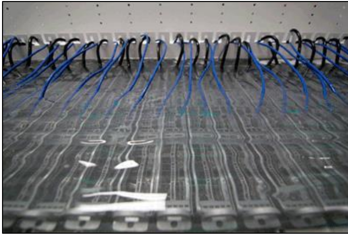
FIGURE 2: IMMERSION COOLED SERVER [15]
