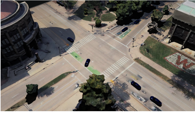
Fig. 5. Second scenario; Vehicles navigating the Park St. intersection by communicating with a traffic light agent that controls the state of the intersection. This represents an urban environment where individual vehicle dynamics are more important.
