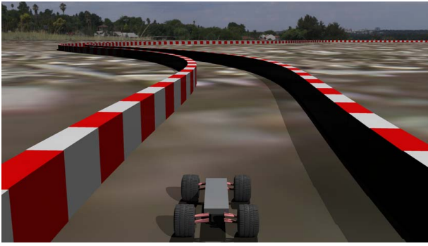
Fig. 12 Demonstration of sensors used to control a scaled autonomous vehicle in simulation. The vehicle uses lidar data to navigate a closed course without prior knowledge of the track.
