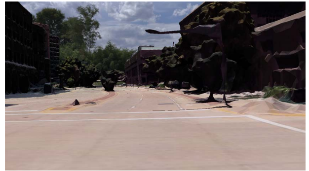
Fig. 16 The front facing camera, in combination with other cameras and lidars, can be used as an input for software-in-the-loop simulation to test autonomous control algorithms
