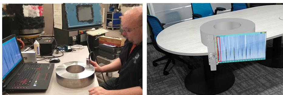
Fig. 1 The traditional hands-on training (left) versus mixed reality training (right) for nondestructive evaluation. The human face and the logos are blurred to protect the confidentiality
