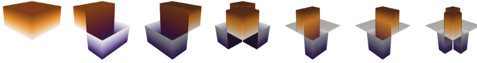
FIG. 12. We recursively divide each panel of \partial\Omega . The basis functions on finer levels are constructed as linear combinations of indicator functions that are orthogonal to functions on coarser levels.
