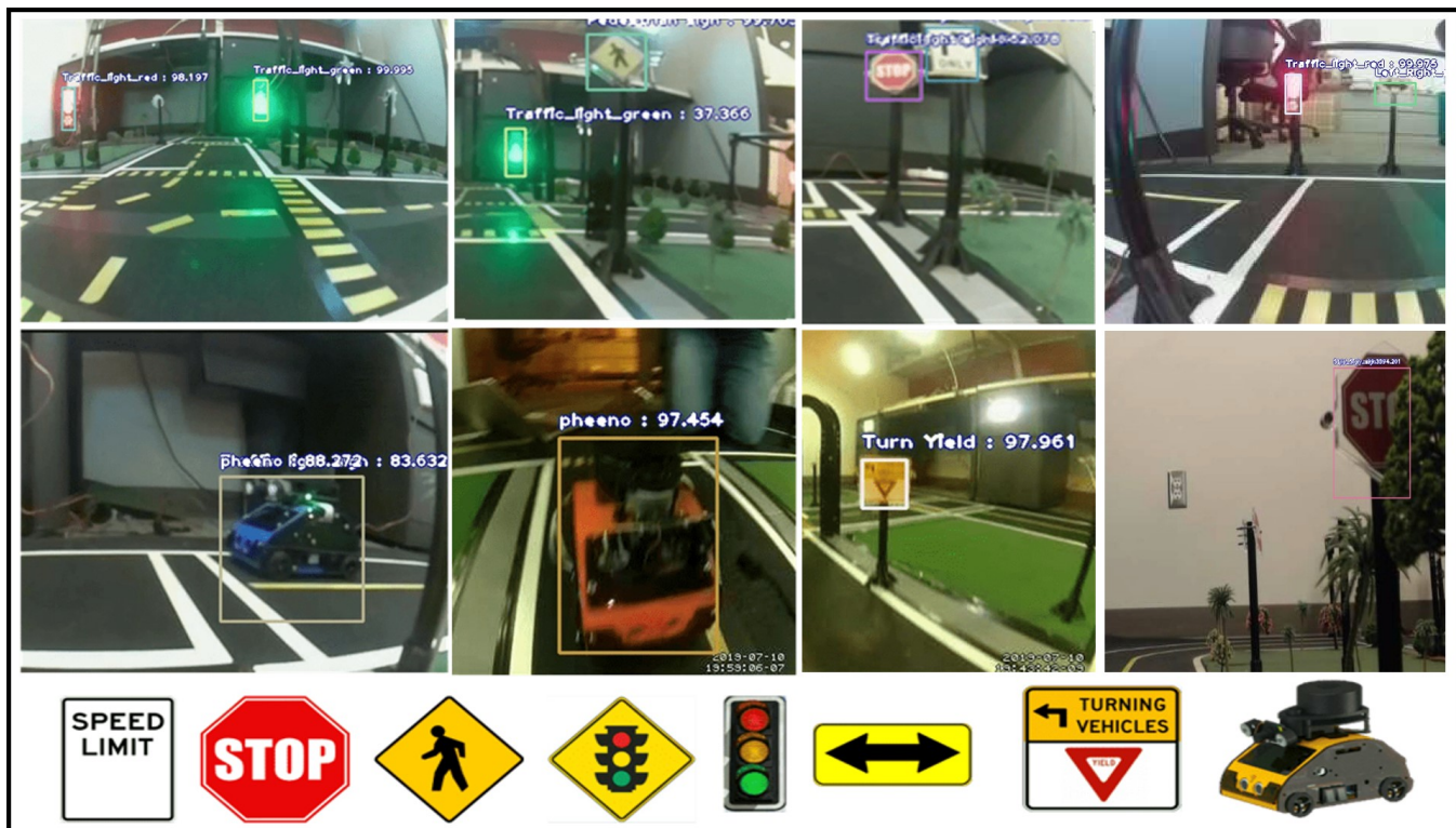
Fig. 7. YOLOv3 object detection results for the video feed from the Go-CHART front-view camera, with bounding boxes and class confidence levels shown. The neural network was trained on the object classes given in the bottom row. Note: The traffic signal includes 3 different object classes: red, yellow and green.
