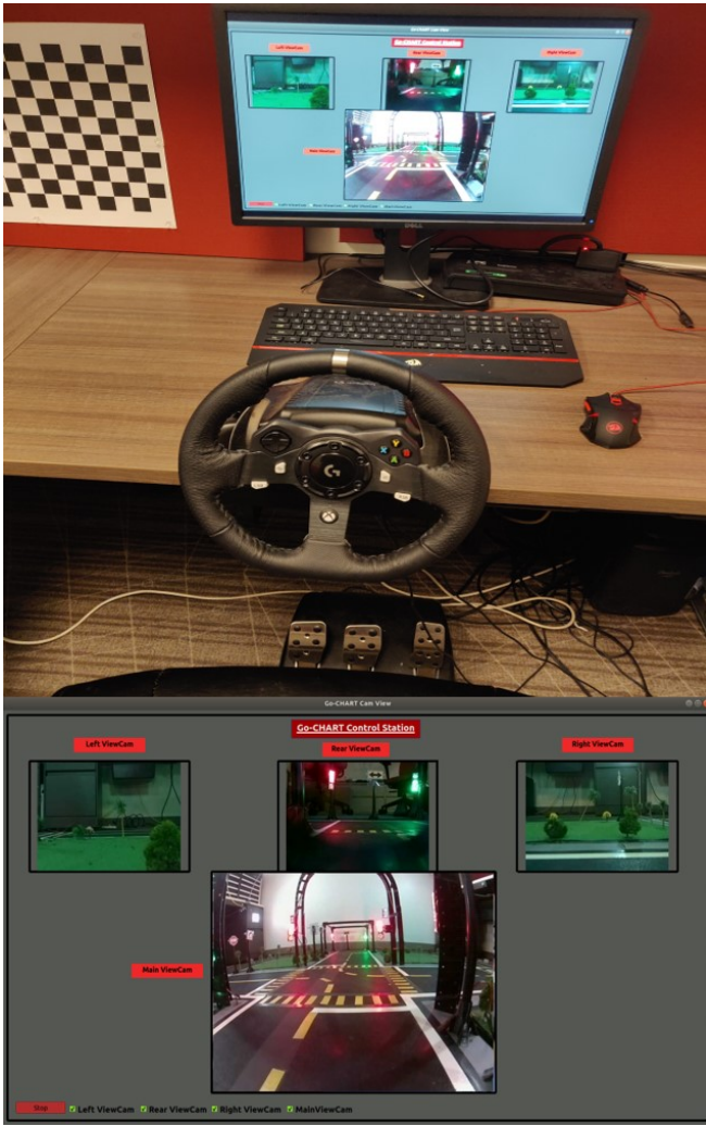
Fig. 6. Top : Driving station setup for Remote-Control driving mode. Bottom : Monitor in the driving station displaying video streams from the front-view, side-view, and rear-view cameras onboard the Go-CHART.
