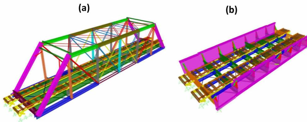
Matlab and the SAP2000 OAPI Open Application Programming Interface (OAPI) were used to automate each type of analysis. Automation was implemented to (i) model selected trains; (ii) simulate damage locations and intensities, of which there were 201 scenarios for the truss and 241 for the through plate girder, for each train passage; and (vi) extract internal effects that included loads (strains), strong-axis rotations, vertical displacements and accelerations.
