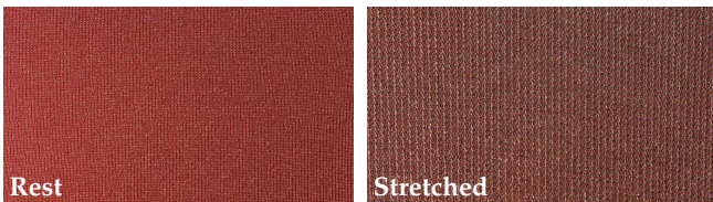
Fig. 2. Appearance change of a real fabric driven by external stretching. When a real piece of cloth is stretched, its internal yarn and fiber structures can change drastically, leading to significantly different overall appearance. In this example, we show photographs of a nylon fabric under rest and stretched states.
