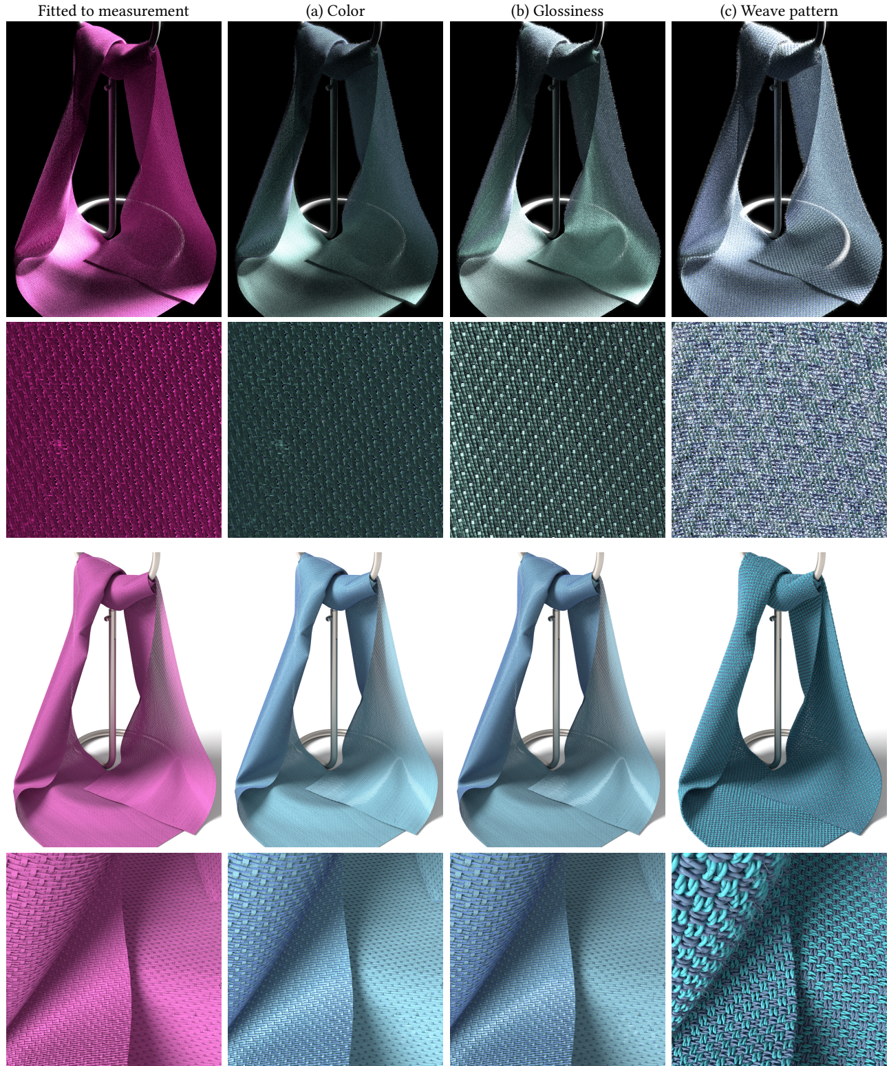
Fig. 13. Editing geometry and appearance. Starting from the Figure 9-b where we use fitted parameters to measurement: (a) Change the color (b) edit glossiness value, (c) change the weave pattern to basket with pronounced flyaways. Note, the subtle appearance of flyaways on the basket pattern which greatly increases realism along the edges.
