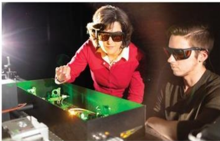
Professor Cheryl Schnitzer and Andrew Fitzgerald (Class of 2021) align a KM Labs Ti:sapphire laser.
