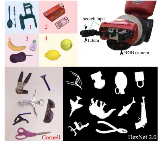
Fig. 7. The robot gripper and the objects used in the robot grasping experiment (top). Some of the objects from the Cornell and DexNet grasping dataset used in the method comparison test (bottom).
