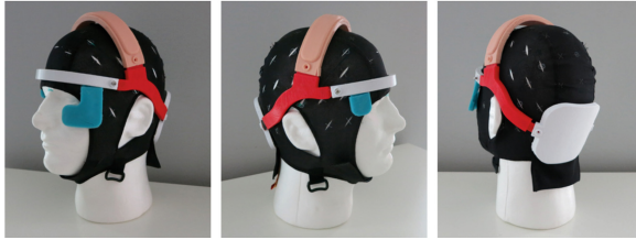
Fig. 6. The prototype on a mannequin head for form and sensor positioning evaluation.
