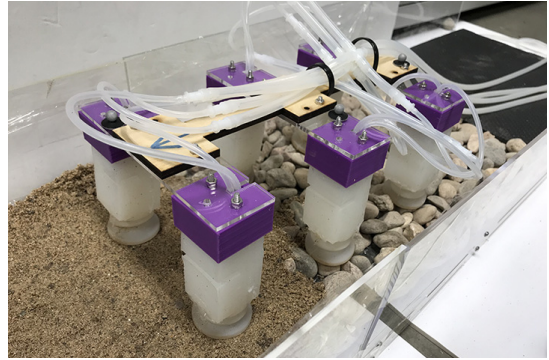
Fig. 1: SoRX, the novel soft legged robot developed in this work. The robot is able to traverse terrains consisting of sand and rocks.
