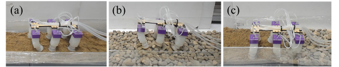
Fig. 14: SoRX was found capable to traverse (a) sand, (b) rocks, and (c) mixed terrain.
