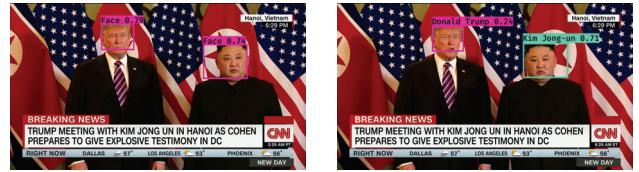
Figure 2: Example Panorama use-case (1): unbounded vocabulary recognition. Left: the frame shows two out-of-vocabulary faces (identities unknown) and the model only labels them as faces. Right: After the user freezes the video, clicks on the bounding boxes and labels them with names, Panorama can recognize these two objects in future frames. The scores shown on the left frame are the probabilities of being faces; on the right frame are the distances from the faces to their nearest neighbor in the Known Objects set.
