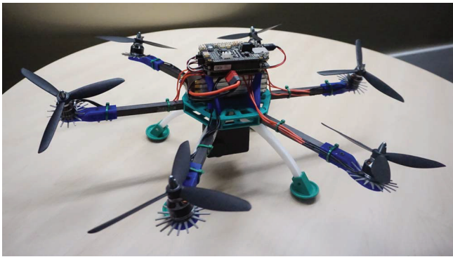
Figure 10. The assembled hexrotor with the optimized rotor configuration from our case study
