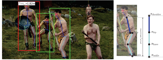
Fig. 6: (Left) Annotated person bounding box (red) with ground truth height and detected person (green) with keypoints (colored). (Right) Calculation of upright ratio.
