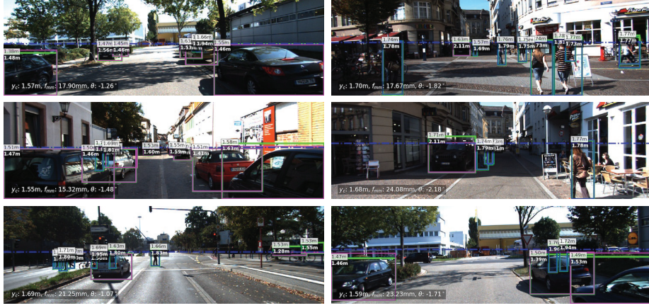
Fig. 9: Scene parameters estimation results with SN-L3-mulCat on KITTI-mulCat. Reprojected pedestrians are in blue, while cars are in magenta.
