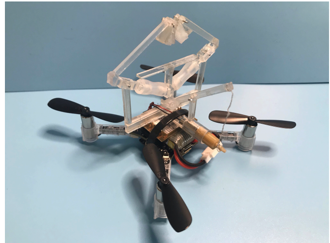
Fig. 8. Perchfly. Gripper is attached to the Crazyflie with a zip tie. The whole system is about 40 g including a flow deck.
