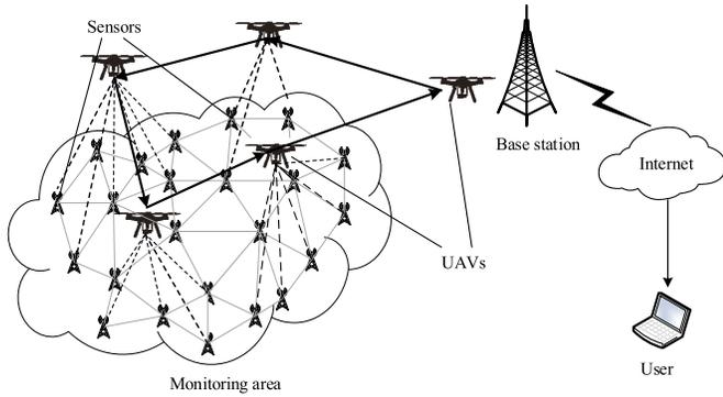
Fig. 1. The architecture of the UAV-based WSN.
