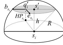
Fig. 4. An example of the flight path  $U_{s_i}$  of UAV in  $\Omega(s_i)$ , which is composed of  $U_{s_i}^f$  and  $U_{s_i}^h$ , where  $U_{s_i}^f = (b_{s_i}, q_i^k) \cup (q_i^k, e_{s_i}^k)$  and  $U_{s_i}^h = (q_i^k, HP_{s_i}^k) \cup (HP_{s_i}^k, h)$ .
