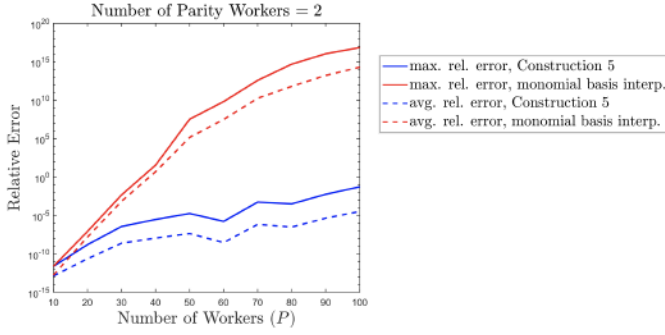
Fig. 13. The growth of the relative error, for Construction 5, using both Chebyshev basis interpolation and monomial basis interpolation, both using Chebyshev points, with the system size given a fixed number of redundant worker nodes equals 2.
