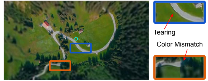
Fig. 2: Foveated streaming of 360° videos requires too many tiles due to the large field of view and high variability of detail. Using too few tiles leads to tearing artifacts (blue box) and color mismatch artifacts (orange box) as shown above. The gaze position is marked with a cyan circle at the center of the frame.
