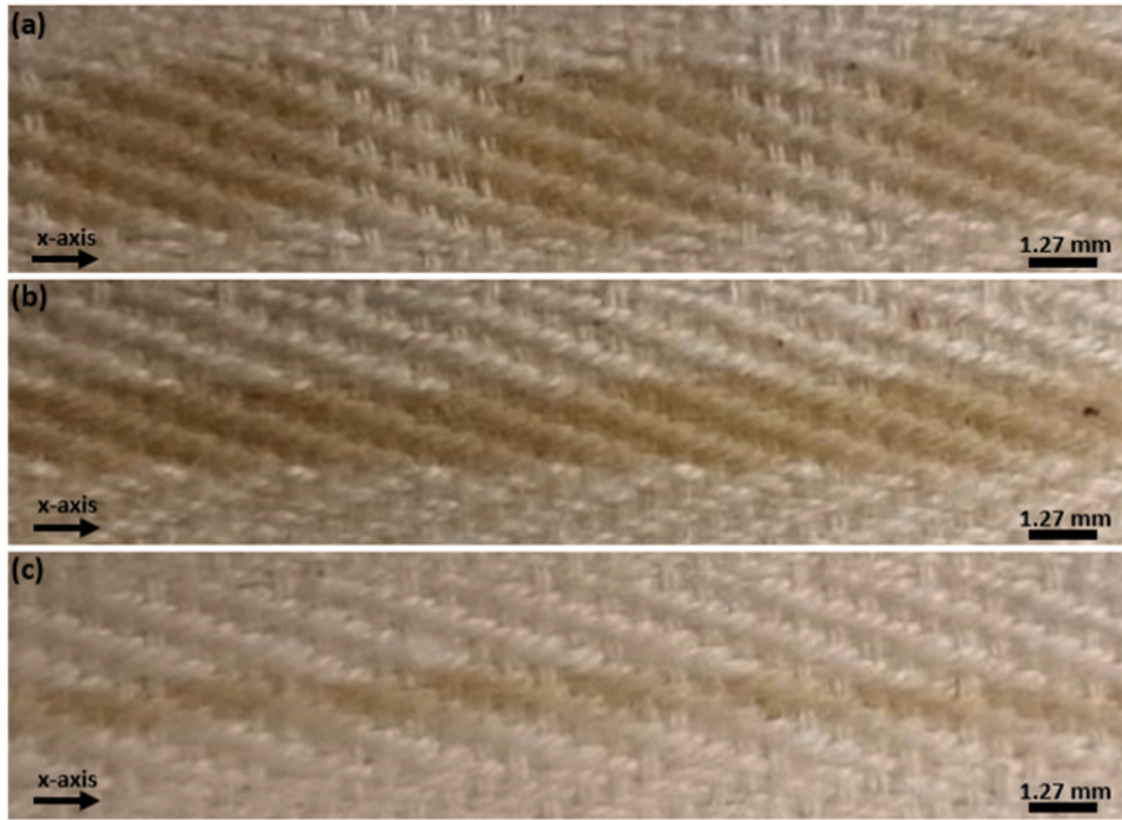
Fig. 16. Spot-E extruded at \sim 29 mm/s from 30-gauge needle onto woven cotton (0.85 mm thickness) adhered with double-sided tape to a glass substrate (1 mm thickness). (a) 0 kV/mm, 40 mm/s, discontinuous trace \sim 3.5 mm wide. (b) 2.5 kV/mm, 40 mm/s, continuous trace \sim 2 mm wide. (c) 2.5 kV/mm, 80 mm/s, continuous trace \sim 1 mm wide.
