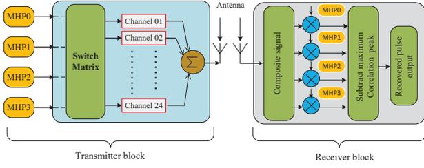
Fig. 2. The functional block diagram of the proposed pulse-encoding scheme based high speed data communication system.
