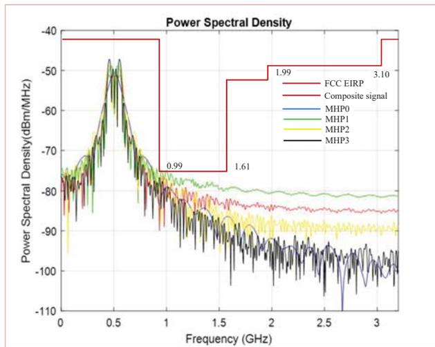
Fig. 6. The power spectral density of the composite signal, MHP0, MPH1, MHP2, and MHP3 after 500 MHz frequency shifting.
