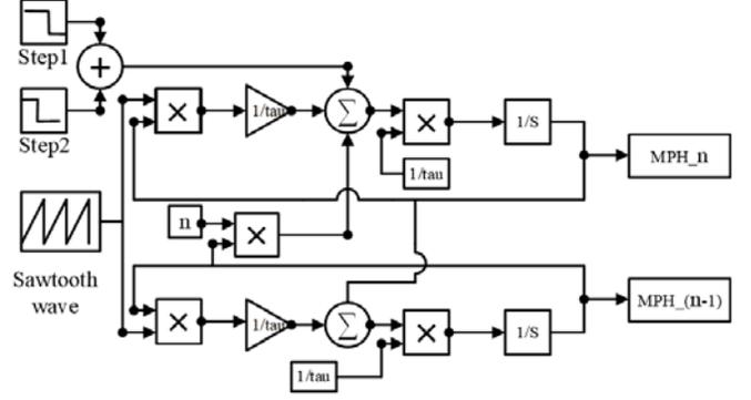
Fig. 3. The Simulink block diagram of the MHP set generator [8].
