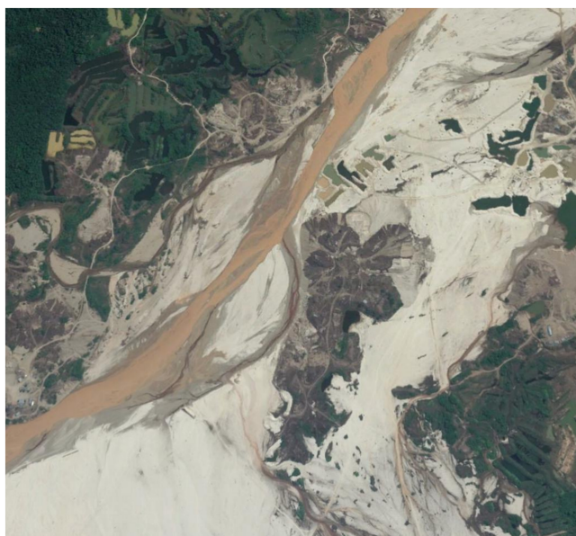
FIGURE 3 Massive siltation impacts along the main channel and floodplain of the Colorado River, Madre de Dios basin, Peru, associated with gold mining operations. Image Google Earth
