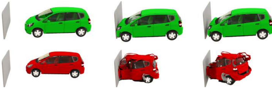
Fig. 8. Simulations of two frontal nonelastic crash scenarios: a car with moderate velocity (top) and high velocity (bottom).
