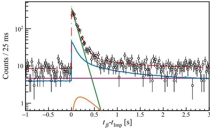
**Fig. 2.** Time distribution of neutron-gated  $^{121}\text{Rh}$   $\beta$ -decay events fitted as part of the analysis. The fitted function (red dashed line) includes contributions of the parent decay (green line),  $\beta$ -delayed neutron emitting daughters and granddaughters (orange line), randomly correlated neutrons (blue line) and a linear random background (purple line).
