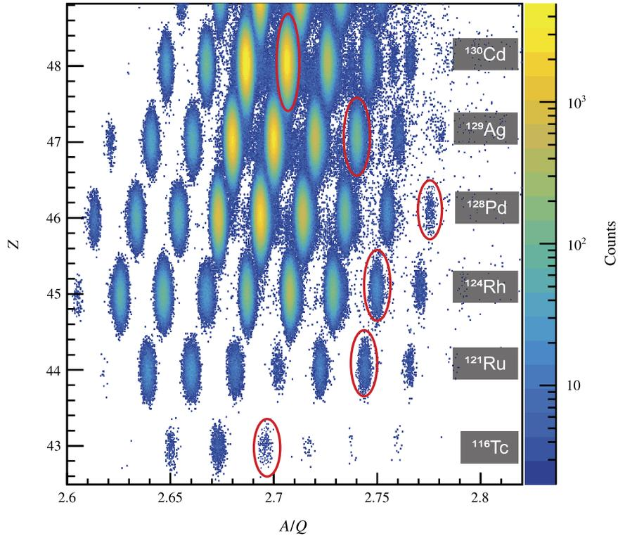
**Fig. 1.** Particle identification plot obtained by BigRIPS showing the atomic number  $Z$  against  $A/Q$  ratio of ions implanted in the AIDA detector stack. Nuclide labels relate to the adjacent groups highlighted by red ellipses.
