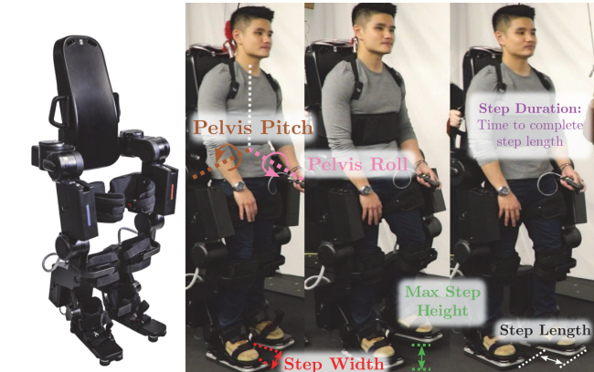
Fig. 1. Atalante Exoskeleton. The exoskeleton has 12 actuated joints. The experiments explore six exoskeleton gait parameters: step length, step duration, step width, maximum step height, pelvis roll, and pelvis pitch.
