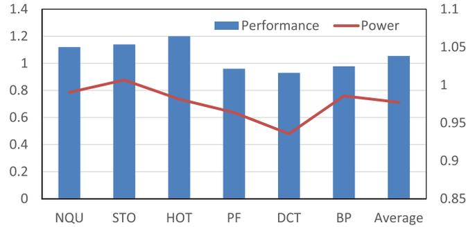
Fig. 15. Overall performance and energy consumption of MLC-based GPU streaming multiprocessor.
