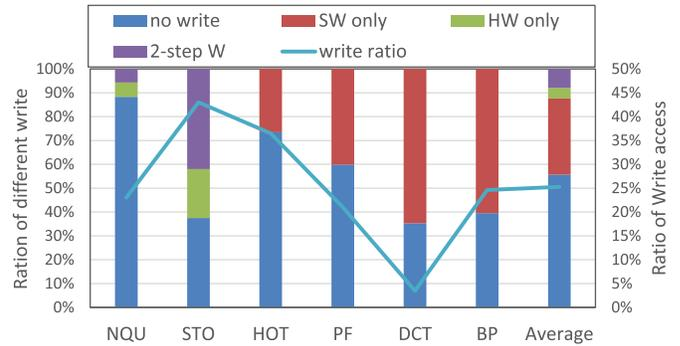
Fig. 6. Actual write bit flip in MLC-STT based shared memory and write access ratio.
