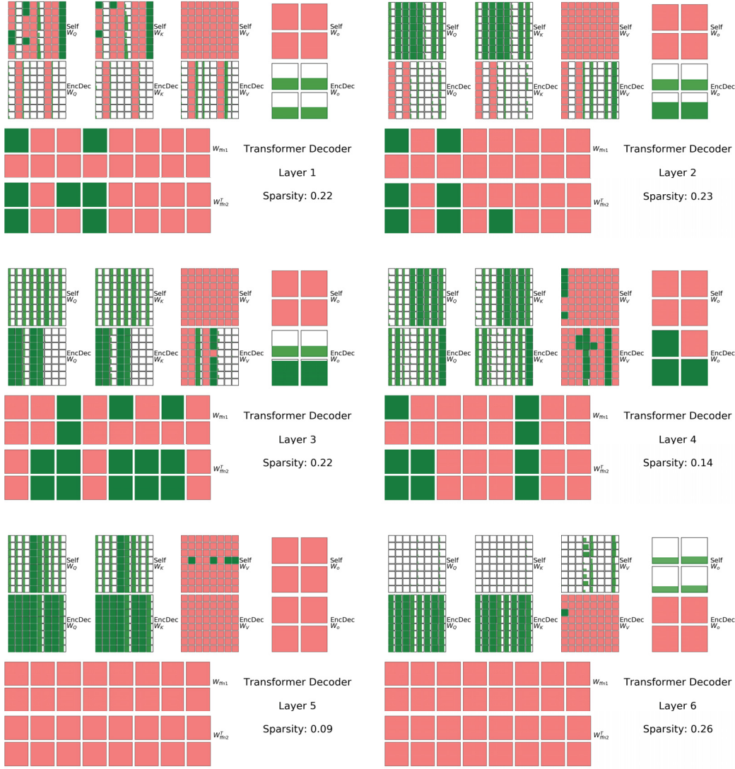
Fig. 6. Sparsity visualization of Transformer decoder with BSSL.
