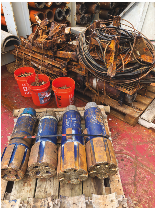
Figure F9. Used mills and recovered wireline CORK materials (i.e., Hole 896A wireline CORK frame on pallets in back, three buckets with junk basket returns), Expedition 385T. Photograph by Beth Orcutt.
