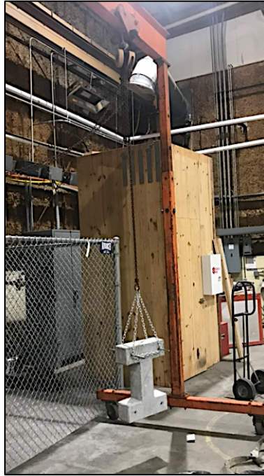
Figure 11: Lifting strategy for tiles using chain hoist.
