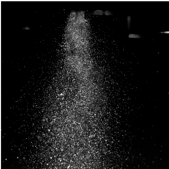
Figure 5. High-speed visualization of the spray exiting the counterflow nozzle as a collection of drops for a water flow rate of 60 ml/min, \beta=0.25 .
