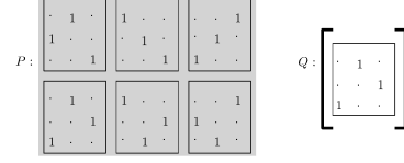
Figure 4: 1D-matching of [19] vs. 2D-matching. Most points in P have frequency = 0, or do not appear in Q . These elements are represented by dots. Each block in P is associated with a unique permutation of (1, 2, 3) . In Q , only one of these 6 blocks appear. Obviously the 2-D data uniquely indicates which blocks of P is isomorphic to Q , and (if only blocks are considered), this block is revealed as the unique optimal solution to the order-preserving matching. On the other hand, the sum of each row and column are identical, so no meaningful 1-D matching is possible. By replacing 3 by an arbitrary d , we indicate that no less than d! false matching are possible.
