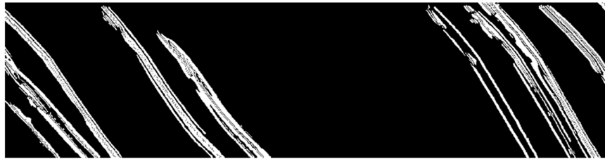
Figure 8. Sample strands detection results using time differencing.
