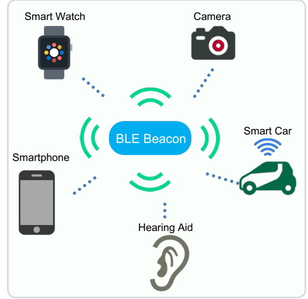
Fig. 1. Different Bluetooth enabled devices receiving BLE signals from the beacon.
