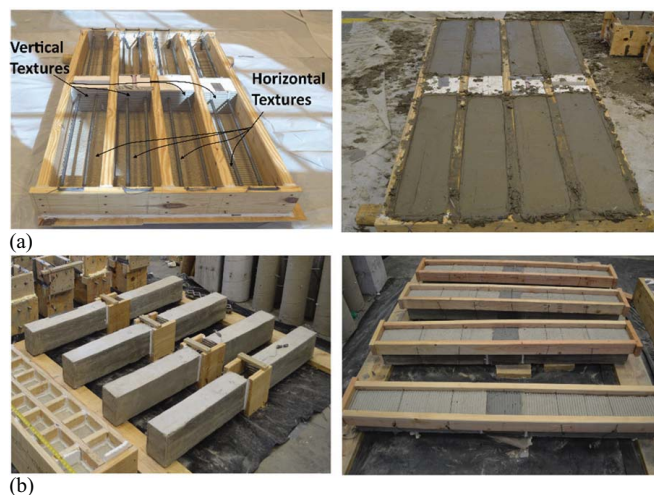
Fig. 3. Specimen fabrication of composite beam specimens: (a) formwork and pouring of NSC; and (b) formworks for pouring UHPC at mid-span and overlay.
