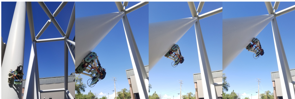
Fig. 25 Adhesive and climbing test on a thin paint-coated steel structure: cylinder shape D=250\text{mm}
