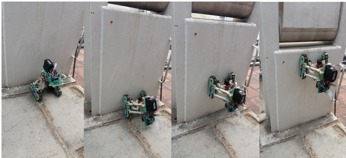
Fig. 23 Adhesive and climbing test on a thick paint-coated steel structure: flat surface
