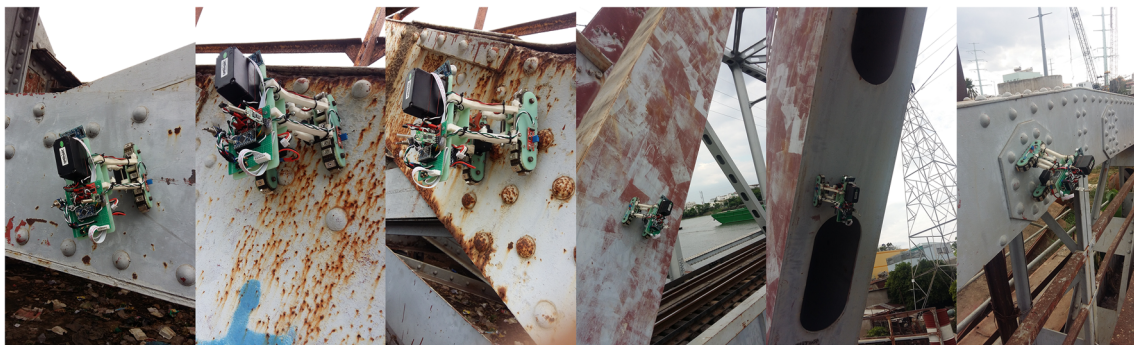
Fig. 27 Adhesive and climbing test on a rusty paint-coated steel bridge: flat structure with bolts/nuts
