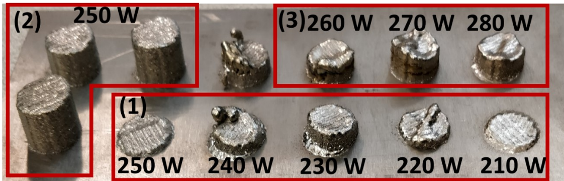
Figure S1. DED processing parameters optimization of pure SS 316L. The designed cylindrical structure had a 0.5-inch diameter and 1-inch height. All samples were fabricated using a hatch distance of 0.417 mm, a constant laser scan speed of 1200 mm/s, and a layer thickness of 0.15 mm. Group 1 was fabricated by a laser power of 210-250 W. Based on the results of the as-fabricated layer, using 250 W to fabricate, SS 316L showed the best result. Group 2 were the cylindrical SS 316L structures fabricated by 250 W. The dimension of the parts from group 2 was closed to the design. Group 3 was fabricated by utilizing laser power from 260 W to 280 W. These parts had a concave top surface, and the as-fabricated parts could not reach 1-inch height, which was caused by high laser power.
