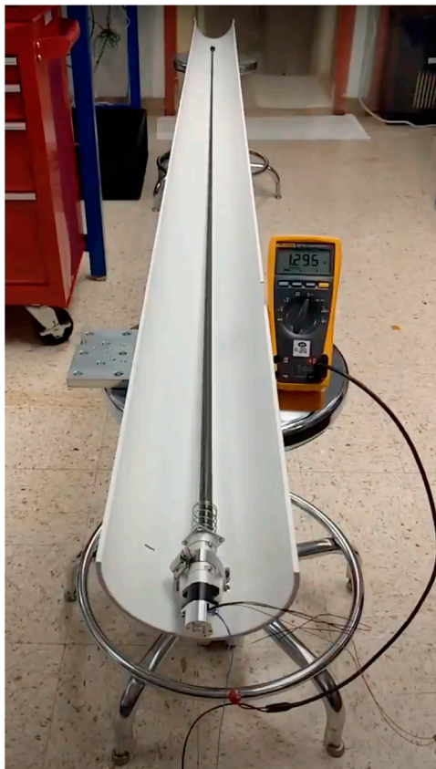
FIGURE 6 | A deployed CURIE stacer antenna undergoing ground testing.
