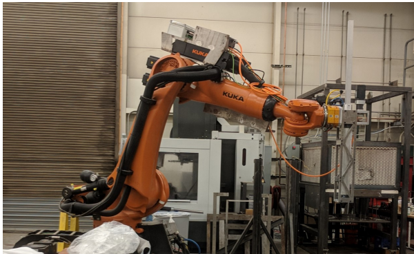
Figure 5. The KUKA KR120 robotic arm for the physical robot module.
