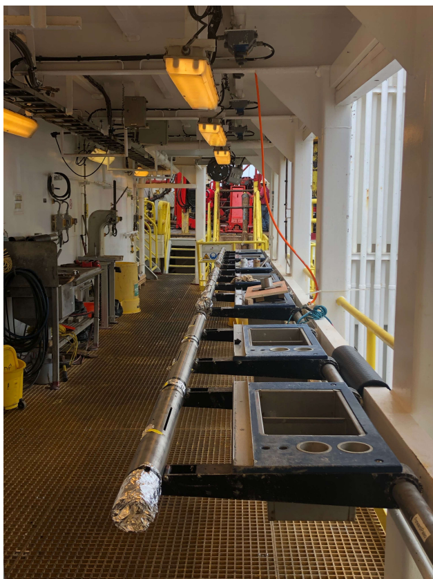
347 Figure 3. Eleven modules were combined in three section on the catwalk in anticipation for 348 deployment within DSDP Hole 504B on IODP Exp. 385T in August 2019 (Tominaga et al., 349 2019). Final assembly and connection to other sensing instruments would occur on the rig floor, 350 which is up the four steps at the end of the catwalk. Aseptic aluminum foil covers the fluid intake 351 to minimize microbial contamination prior to deployment.
