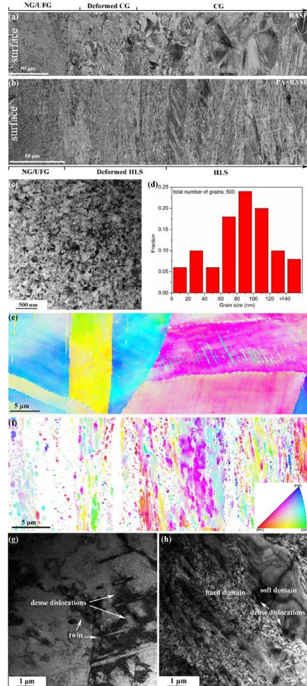
**Fig. 2.** Representative microstructure starting from surface (a) RASP and (b) PA+RASP samples; (c) and (d) TEM image of the nano/ultrafine layer of PA+RASP samples ( $< 30 \mu\text{m}$ ) and grain size statistic of the nano/ultrafine layer; EBSD image of (e) RASP and (f) PA+RASP at depth  $\sim 100 \mu\text{m}$ ; TEM image of (g) RASP and (h) PA+RASP at depth  $\sim 100 \mu\text{m}$ .
