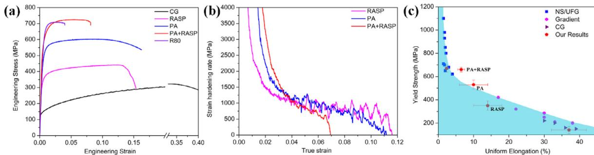
**Fig. 1.** (a) Strain-stress curves of the samples fabricated by different processing routes; (b) Strain hardening rate curves of the samples; (c) Comparison of mechanical properties of brass samples with different structures [25–29].
