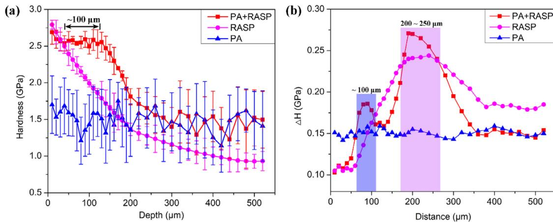
**Fig. 3.** (a) Hardness profile of three different samples; (b) Increment of hardness after 3% of tensile plastic deformation (the shaded area indicates the peak of the hardness profile).
