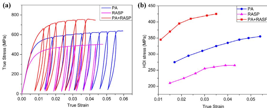
**Fig. 4.** (a) Loading-unloading-reloading (LUR) test to measure the HDI stresses. (b) HDI stress calculated from the LUR curves.
