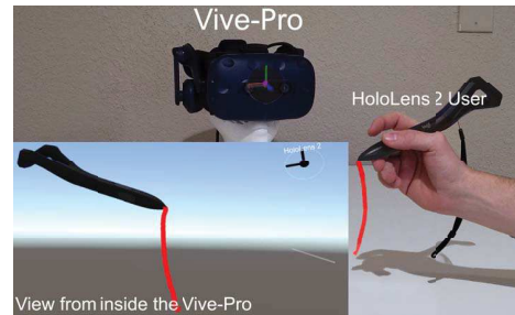
Figure 3: A HoloLens 2 user drawing a line using the VR-Pen as seen by both the HoloLens 2 user and the Vive-Pro user
