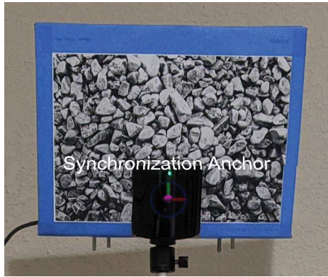
Figure 1: Vuforia image target mounted on top of Vive-Pro Base Station 2.0, synchronization anchor position adjusted down from the center of the image target to the base station center.
