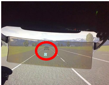
Figure 4: Representation of the secondary glance task paused on the letter H. Red circle represents a possible glance concentration effect.
