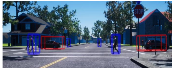
Figure 1: AR cues conformal bounding boxes concept used in this work: blue bounding boxes to highlight pedestrians, red for vehicles.
