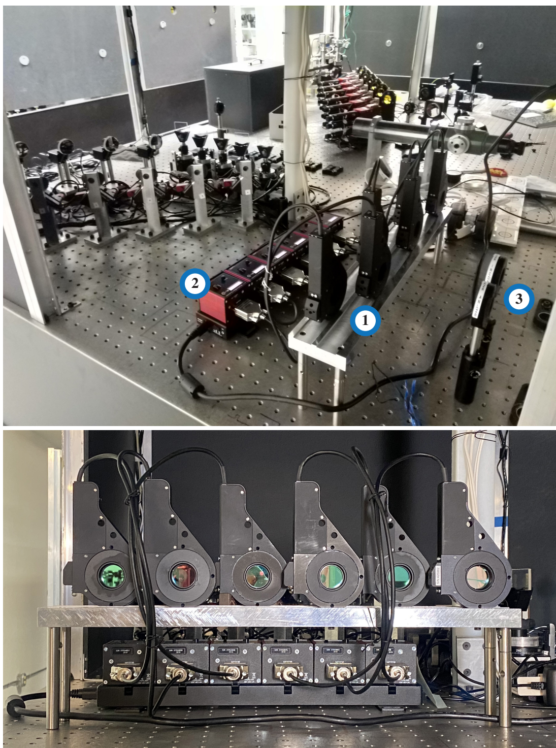
Figure 2. The new polarimetric hardware installed on the MIRC-X optical bench at CHARA. The top panel shows the half-wave plate assembly ① and motor control boxes ② in relation to the MIRC-X instrument during initial testing in 2019 November, where calibration was conducted with a pair of linear polarizers ③. Not pictured is the mini-PC, which is installed above the MIRC-X table, controlling the motor boxes via USB. The bottom panel shows the waveplates “beam-on” during on-sky observations in 2020 November.
